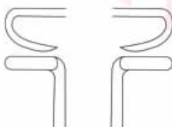
Killian Septum Elevator, Double Ended, 4 mm With 3.4 Mm Taper, And 4.3 Mm With 3mm Taper, 09-083 184mm Length
